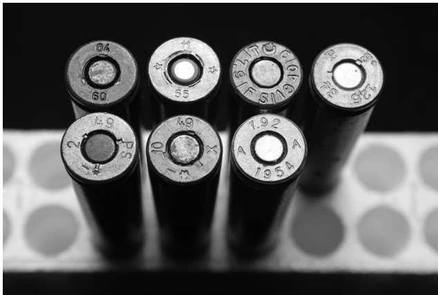
Figure 3.9 (See color insert.) The 7.92×57mm cartridge remained popular even after the Second World War, and production continued because of its widespread use around the world and the large amount of surplus German arms in circulation. Top row from left: East Germany Factory 04 (1960); Prvi Partizan, Yugoslavia (1955); Kirikkale/Ankara, Turkey (1940); and prewar German production (1934)—note P126 code. Bottom row from left: Two variations of Czechoslovakian production by Povazske Strojarnje/Povazska Bystrica (late 1940s); and Ammunitions Arsenalet Denmark (1954), often called the 8mm Mauser. (Image from author’s collection.)
